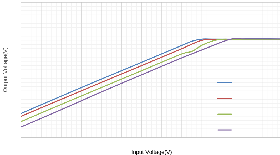
Figure 10. LDO Operation Characteristic ( V_{OUT}=5V )
