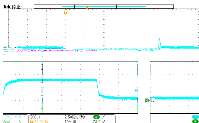
Figure 39. DC-DC Load Transient (10mA-150mA), V_{OUT}=5V
