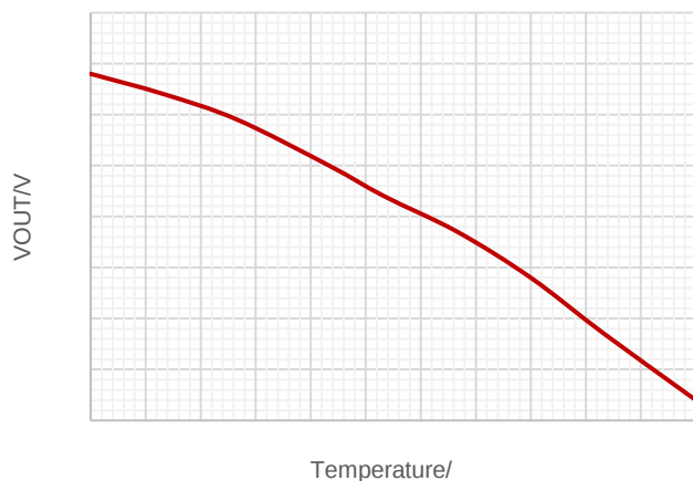
Figure 5. Output Voltage vs Ambient Temperature at VOUT=5V
