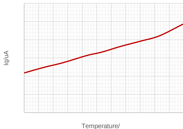
Figure 3. Quiescent Current vs Ambient Temperature
